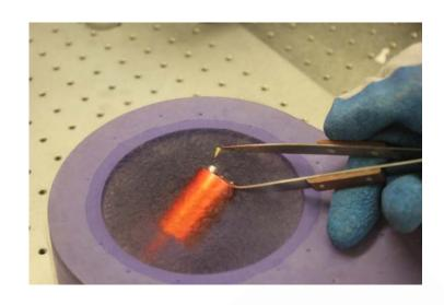
2: Lift the Ice-off out of the LN2 with vent at upward position. The best working angle of the Ice-off is nozzle point down at 10° to 45° angle as show in figure on left.
