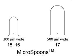
Push, detach from surfaces, separate from a cluster, lift, transfer Push down to flatten tip and slide under sample.
