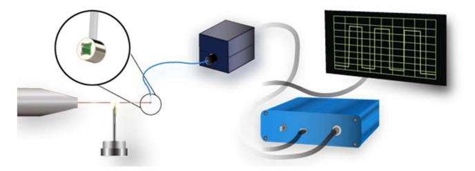
A housing forms the beamstop and the scatter shield around the heart of the Sentinel device. A beam reducer or collimator is not used and is not formed as part of the beamstop. The Sentinel device is attached by the user to a beamstop blade produced by the user. The device signal is coupled into and travels down the fiber optic cable, which connects to the Diode-Cable Assembly.
