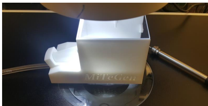
The Humidified Sample Workstation in position on a stereomicroscope with a large working distance.
