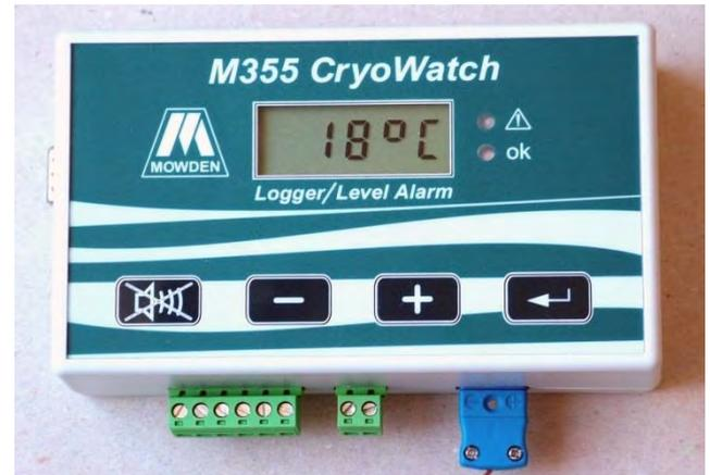
The M355 also stores a record of temperature for verification of correct storage conditions. The Interval between measurements is adjustable between 1 minute and 30 minutes.
