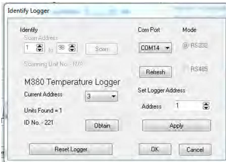
If this is the first use of the software it may be necessary to select the required COM Port from the pull-down menu and click on the '*Obtain*' button to identify the Logger. The program should default to this setting on subsequent use of the program.
