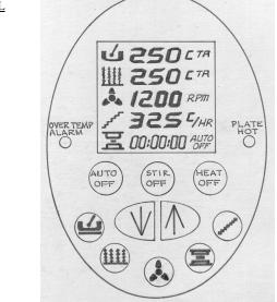
Shown above are the keyboard and display for the HS30 Digital Hot Plate/Stirrer.
