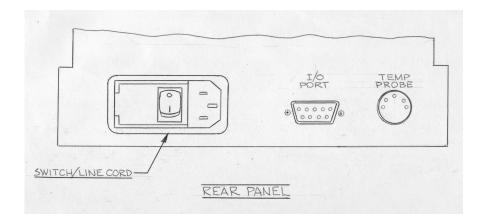
The AC power connector jack, fuse holder and switch are a module mounted on the right rear of the unit. The temperature probe jack is mounted to the right. Note the polarity on the probe jack. Be sure not to force this connection when plugging in the temperature probe.
