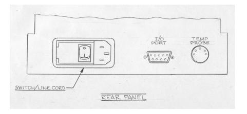
The AC power connector jack, fuse holder and switch are a module mounted on the right rear of the unit. The temperature probe jack is mounted to the right. Note the polarity on the probe jack. Be sure not to force this connection when plugging in the temperature probe.
