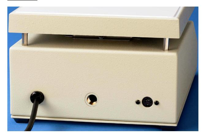
Shown are the AC line cord, input fitting for the purge port, and probe connector jack. The AC line cord is a three-wire grounded cord. The fuse is inside the unit in an inline jack on the hot side of the AC input. The fuse type and value appear on the label on the rear of the unit. The gas fitting is a ¼" NPT 18 threads per inch 0.40 thread engagement fitting. Be sure to use dry inert gasses only.
