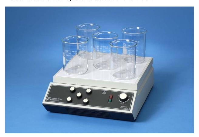
On the **9-position** stirrer, the pattern of stirrer controls is from the lower right to the upper left in 3 slanted rows. The right row of knobs/controls from bottom to top is for the stirrer positions on the right side of the heater top from front to back. The center row of knobs/controls from bottom to top is for the middle stirrer positions from front to back. The left row of controls/knobs from bottom to top is for the left side of the heater top from front to back.
