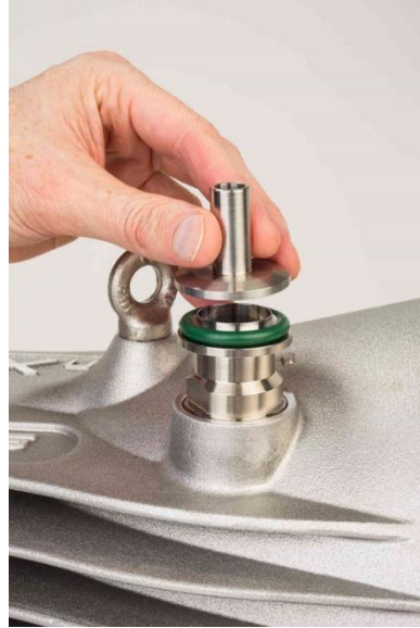
(B) • Inlet port adaptor on centering ring
