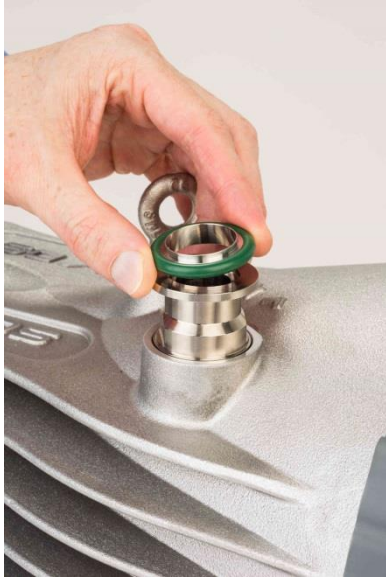
(A) • Centering ring on pump inlet
