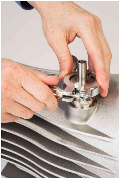
(C) • Swing clamp around inlet port adaptor
