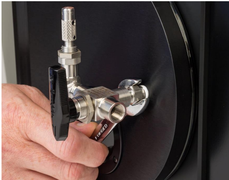
FIGURE 4 • Connecting the Metering Valve/3-Way Valve to the Plasma Cleaner Door
