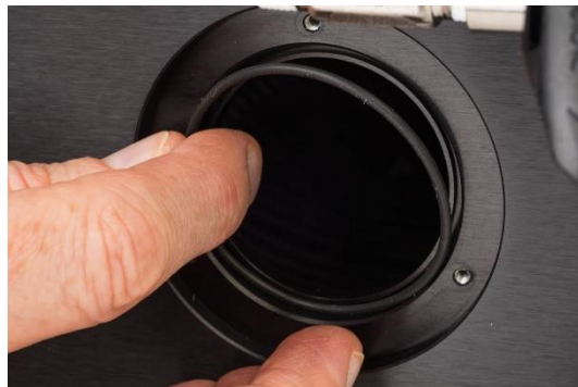
FIGURE 18 • Replacing the Window on the Plasma Cleaner Door
