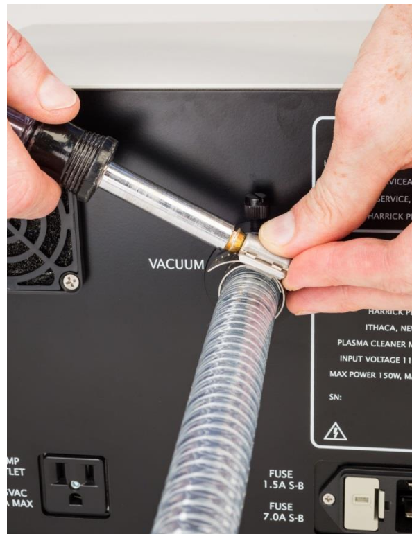
FIGURE 5 • Connecting the Vacuum Hose to the Plasma Chamber Outlet
