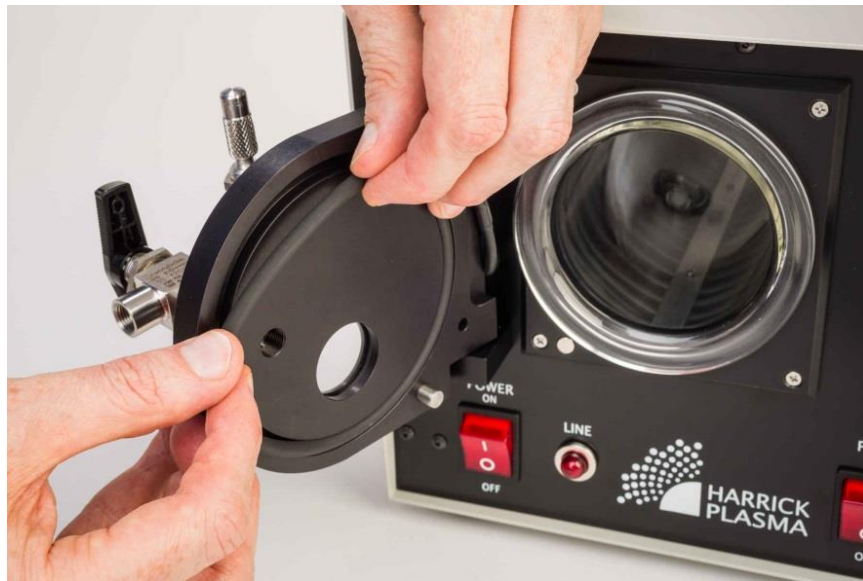
FIGURE 17 • Removing the O-Ring on the Plasma Cleaner Door
