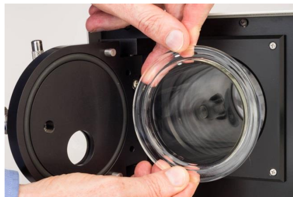
FIGURE 16 • Replacing the Plasma Chamber
