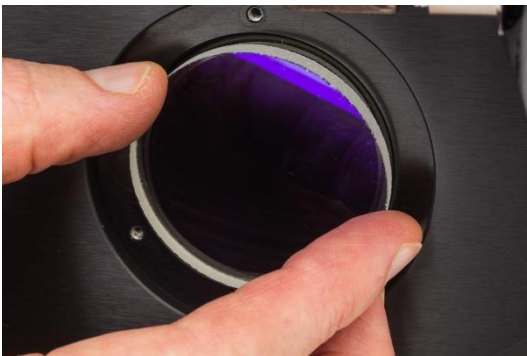
FIGURE 18 • Replacing the Window on the Plasma Cleaner Door
