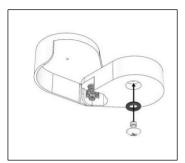
Specimen Preparation: Place the specimen onto the holder, and secure using any tape of choice.
