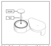
3. Shuttle Sealing: Rotate the lid of the shuttle until it is closed. Align the hand pump with the check valve on the lid of the shuttle, and operate the pump while applying downward pressure onto the lid. A mild vacuum is generated within the shuttle after a few strokes of the pump. Protection of the air- sensitive specimen is effective for up to 24 hours.
