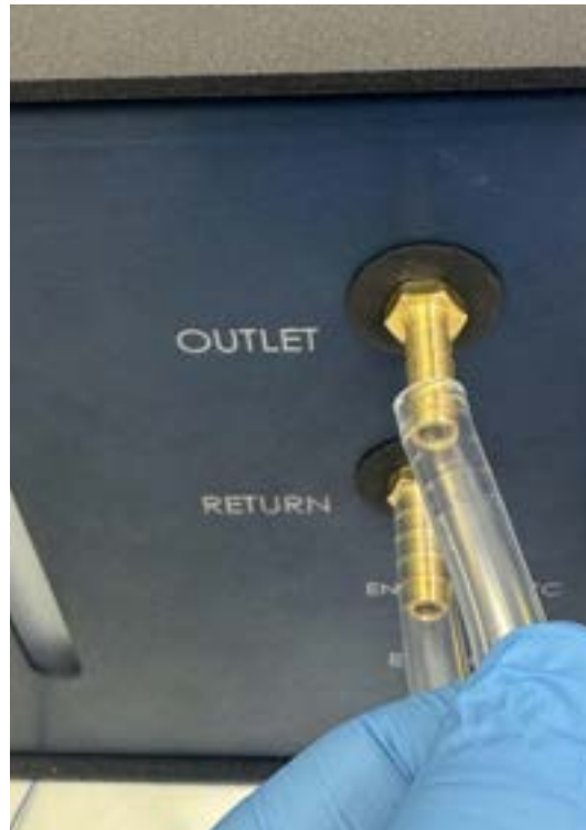
Figure 5: Coolant line connection to front panel of chiller unit
