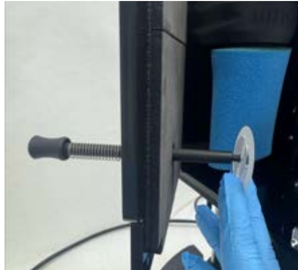
Figure 9: Correct assembly of blotting round and blotting rod through the enclosure side door
