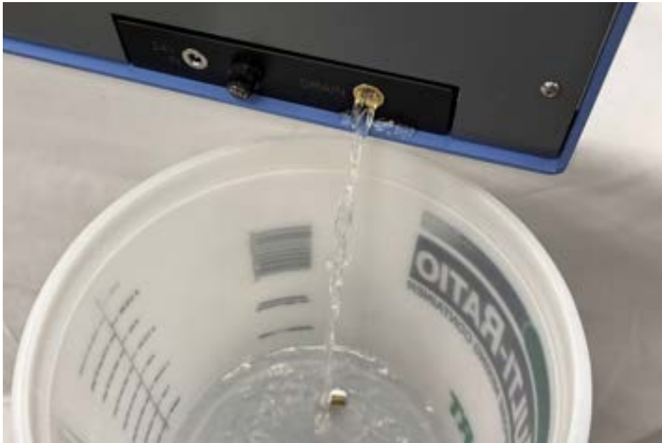
Figure 14: Draining coolant from cooling system
