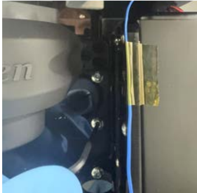
Figure 3: Assembly of Gravitri 4C enclosure and stem by three M4 screws
