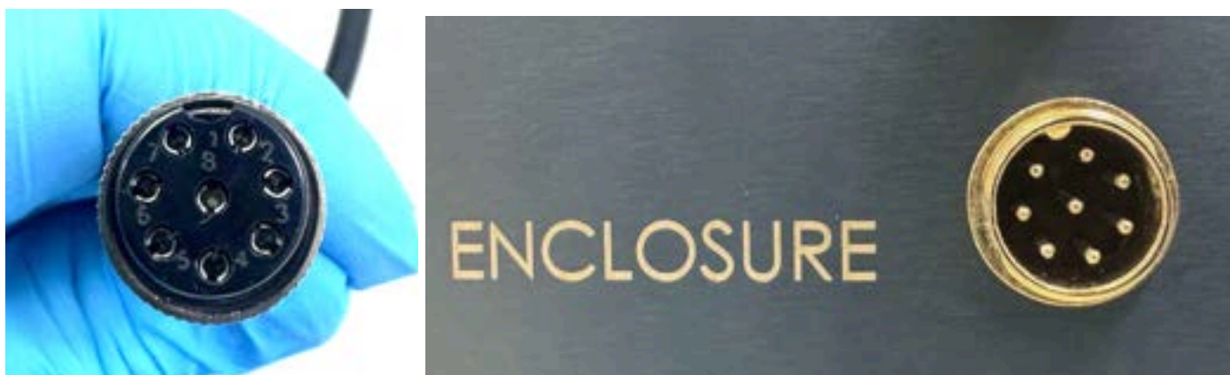
Figure 7: 8-pin connector from enclosure (left) and complementary socket on front panel of chiller unit (right). TAKE NOTE OF THE SEMICIRCULAR LOCATING FEATURES AND ALIGN THEM BEFORE APPLYING FORCE AND SCREWING THE THREADED FASTENER
